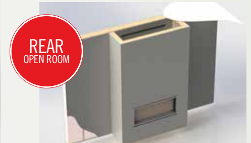
This style of enclosure includes an air outlet opening that will be built into the rear of the constructed enclosure, at the top, centered above the appliance.
